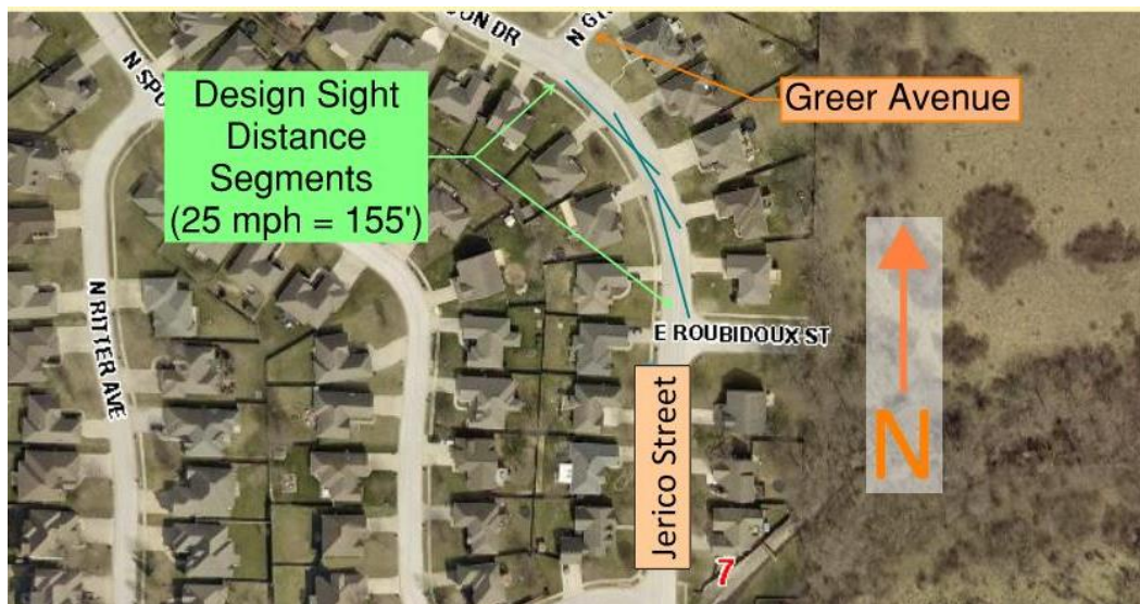
Figure 2: Horizontal Lines of Sight (Design) – North End
