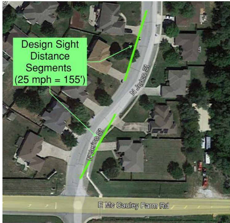
Figure 3: Horizontal Lines of Sight (Design) - South End
